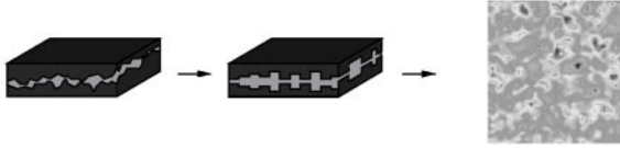
Figure 6: Approximation of rough fractures by parallel plates.
